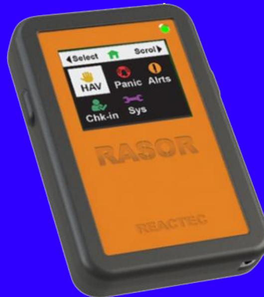
**R-Link** and **RASOR** work with the Reactec Analytics to report exposure data and support optimisation of controls to reduce risk ALARP.
