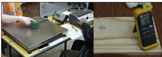
Fig. 3. TTS assessment using vibratory sensation meter (Rion Company Ltd. Model AU-02A) and skin temperature measurement apparatus using thermocouple sensor (RS 206–3738).
