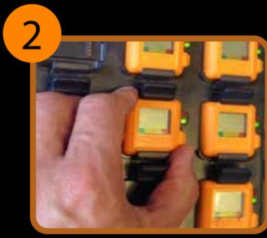
2. Unclip the HAVwear from the bay with the flashing LED light
