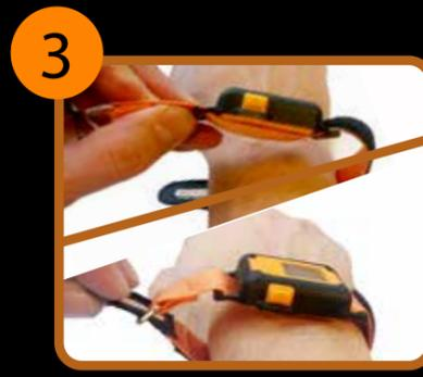
3. Insert HAVwear into the holder so that the strap is in contact with the wrist. Snugly fit the strap around the wrist (do not remove until returning to a Docking station).
