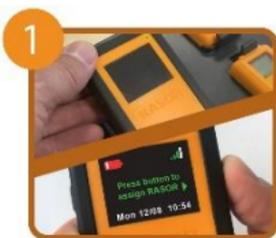
1 Remove the RASOR from the charger and the screen will display the need to assign the RASOR to a user by pressing the right hand button.
