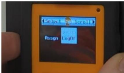
If you have a Dual Charger, you can simply dock the RASOR back into the Dual charger then press the LH button to log off.
