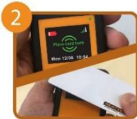
2 The screen displays an instruction to place a valid ID card onto the screen area. Once placed, remove the ID card when a beep sounds to confirm the RASOR has been assigned.
