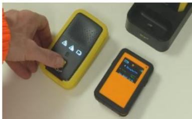
*Press the LH button on the RASOR to scan for the XD1+*
