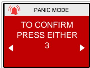
Press and hold both buttons for 3 seconds
