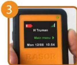
3 After assignment the screen will display the users first name and the option to select the button to view the main menu.
