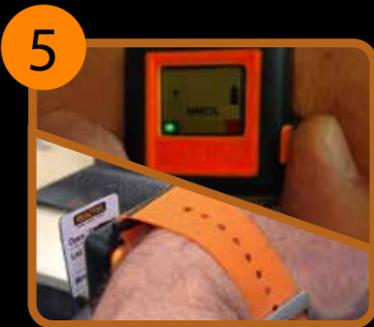
**5.** To "connect" to a SAFE-ZONE press the button on the HAVwear once, place the HAVwear over the SAFE-ZONE tag until a beep sounds. The display will show "SAFE" to indicate social distance detection is switched off.
