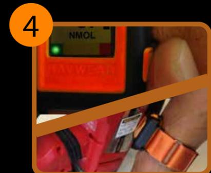
**4.** Before using each tool, press & release the HAVwear button once and place the HAVwear over a tool tag until a beep sounds, to "Connect" to the tool. The display will show the last 4 characters of the tool ID to confirm connection.
