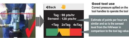
\*Note the reading is updated approximately once a second and is not a rolling average over the time since activation. This contrasts with instruments designed to measure vibration dose which average the dose from the start of the test and do not allow for real time analysis of technique.
